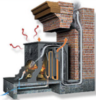
Figure 1.2: Franklin stove, an advanced fireplace with improved heat transfer capabilities invented by Benjamin Franklin in 1742. Source: The Amazing Adventures of Ben Franklin [11].
