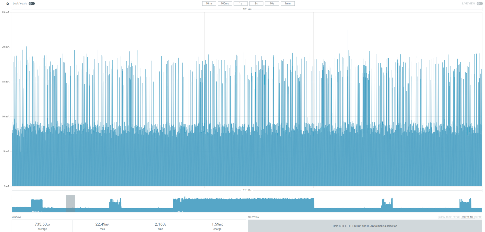
Figure B.1: Low power segment of the wireless station power profile (segment 1 of 2).
